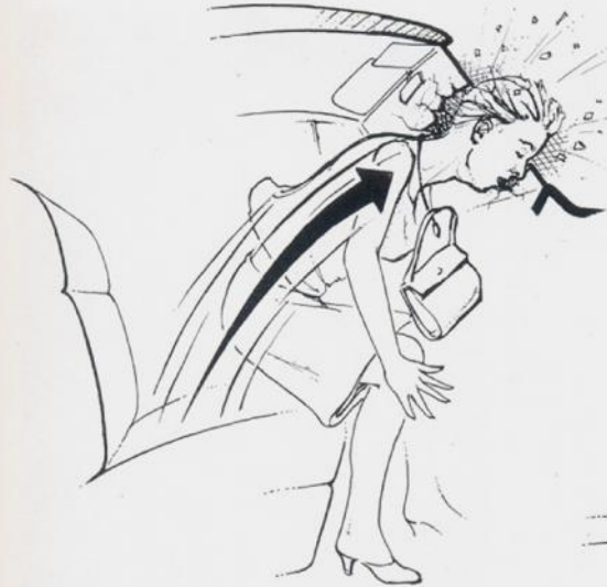
A Passenger thrown up and forward through windshield
